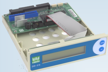
Wytron DVD-319 1 to 3 DVD Duplicator controller. Ideal for cost effective, low volume DVD replication.
