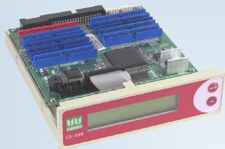
Wytron CD-398 1 to 9 CD duplicator controller. Build your own professional CD replication systems.
